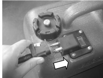
2. Connect fuel joints securely and squeeze the primer pump with the outlet end up until you feel it becomes firm .
