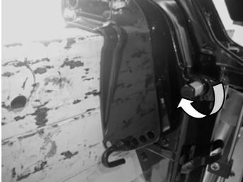
3. Disconnect the fuel line from the outboard motor.
