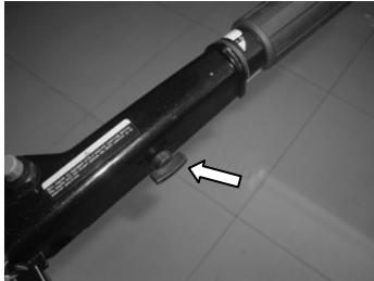
The throttle friction adjuster is on the tiller handle, which provides adjustable resistance to movement of the throttle grip, and can be set according to operator preference. To increase resistance, turn the adjuster clockwise. To decrease resistance, turn the adjuster counterclockwise. When constant speed is desired, tighten the adjuster to maintain the desired throttle setting.
