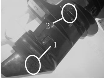
1. Gear oil drain screw
