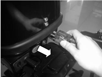
4. Tilt the engine up fully until the tilt support lever automatically locks.
