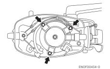
4. Insert the knotted end of the starter rope into the notch in the flywheel and wind the rope clockwise around the flywheel several turns.
