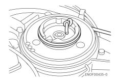
5. Tie a loop in the another end of the emergency starter rope and attach socket wrench, Both the loop and the wrench are provided in outboard motor box.
